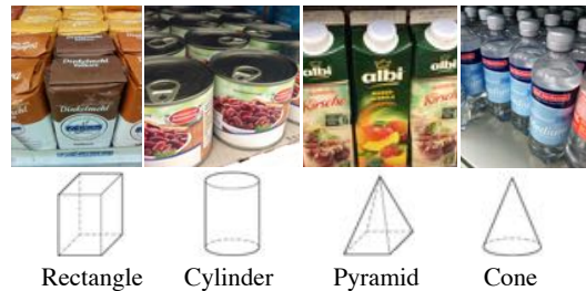
Fig. 2. Main product shape categories, that comprise 90.1% of items in the dataset, are defined based on the the shape of their base and their tip. The shape of the tip determines whether the objects can be stacked or not. The shape of the base determines whether the object is more compactly arranged on a regular grid (rectangular) or an off-grid arrangement (circular).
